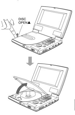
4 Load a disc with the label side up and push down around the center of it.
